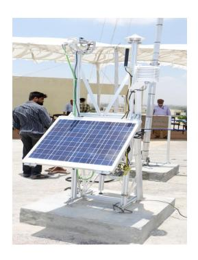
The weather station is capable of observing multiple parameters including solar irradiance, temperature, relative humidity, air pressure, wind speed
