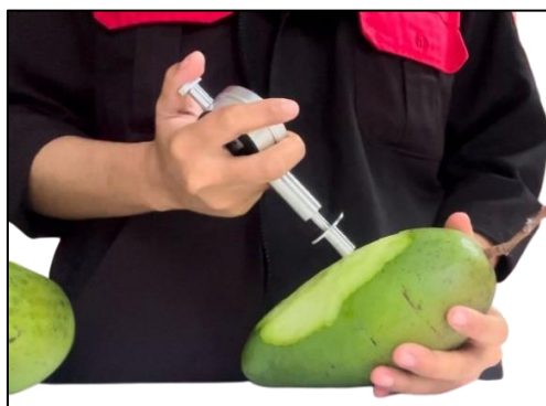
Figure 7. Firmness measurement using a GY-03 sclerometer for farm hardness
