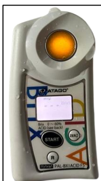
Figure 6. Measurement of Soluble Solid Content using a digital refractometer
