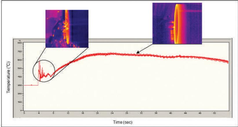
Figure 4. Maximum pin temperature measured during the rubbing process, using the thermal imaging camera
