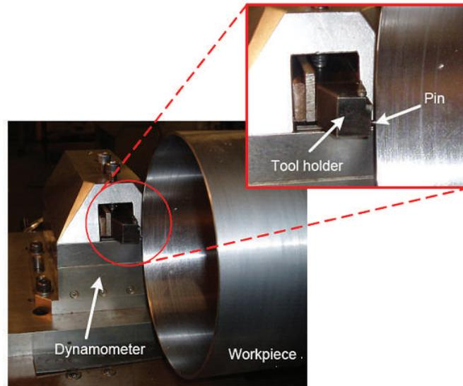
**Figure 1. Experimental setup for the pin rubbing tests**
