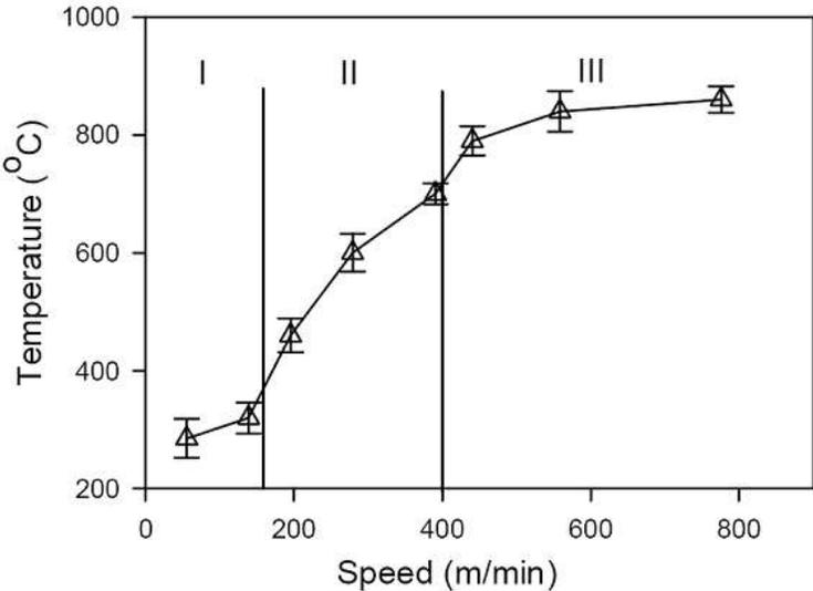
Figure 5. Variation of pin temperature with cutting speed
