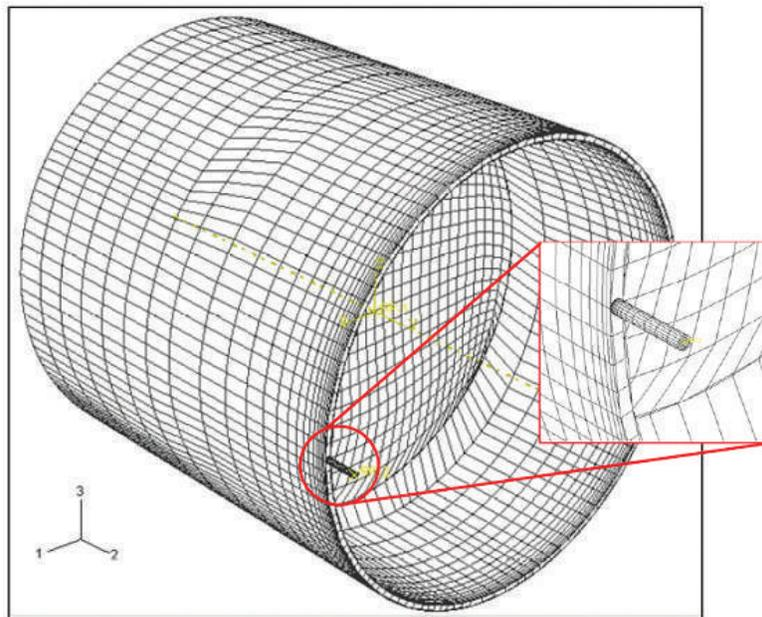
**Figure 9. FE model of the rubbing process**
