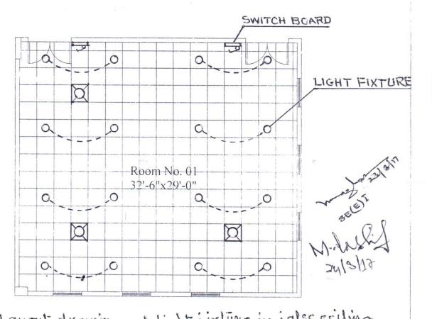
DRG.NO 02 Layout drawing of light fixture in jales eciling
